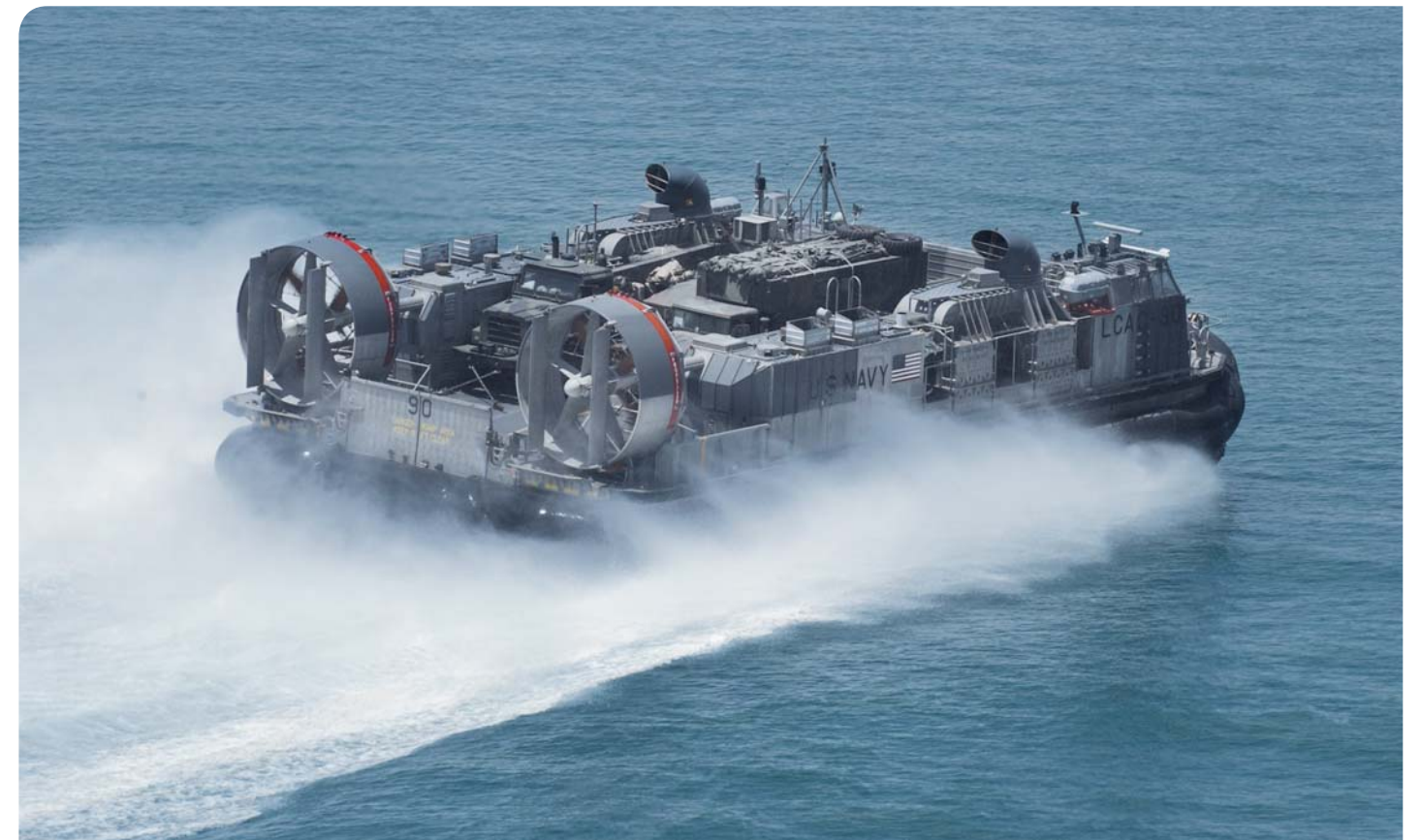
The U.S. navy's Landing Craft Air Cushion (LCAC) uses four TF series gas turbine in each craft.
