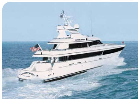
The mega yacht "Detroit Eagle" uses one TF50 in a center boost configuration.
