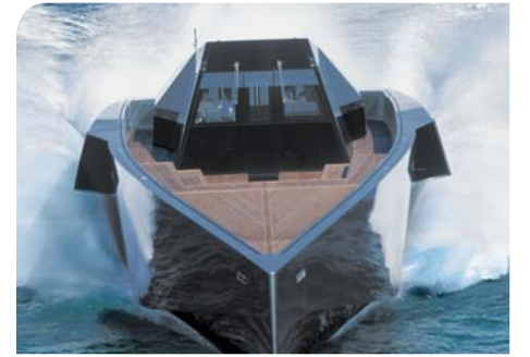
The Wallypower 118 is powered by three Vericor TF50 gas turbines.
