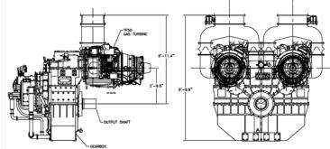
The Twin Package can be configured with the engines side-by-side or with the engines mounted one over the other in a Vertical Twin configuration. This allows adaptation to a variety of hull forms including catamaran and trimaran.
